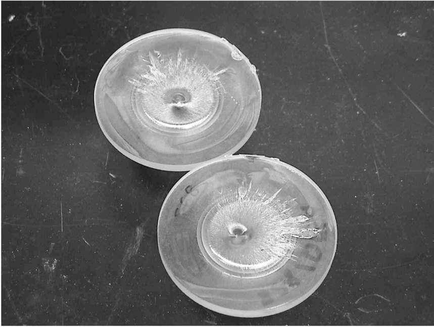
FIGURE 13 Photo of a failure surface in a tensile ramp tests at -10^{\circ}\text{C} .
