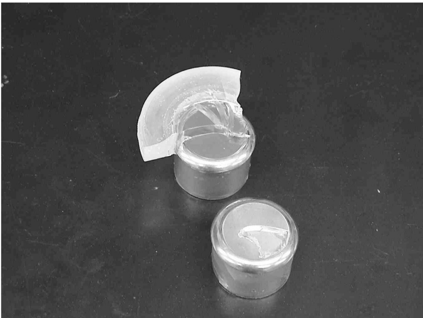
FIGURE 16 Photo of a failure surface in a torsional ramp test.
